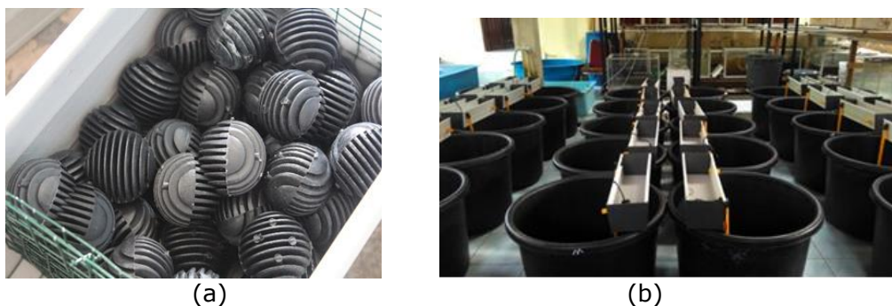
Figure 1. (a) Bioball used as a filter substrate, (b) The design of the Trachinotus blochii aquaculture recirculation system (original).
